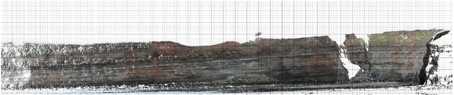
Figure 3. Example of data captured from the cliff top scanner. White areas are occluded (invisible from the scanner position).
